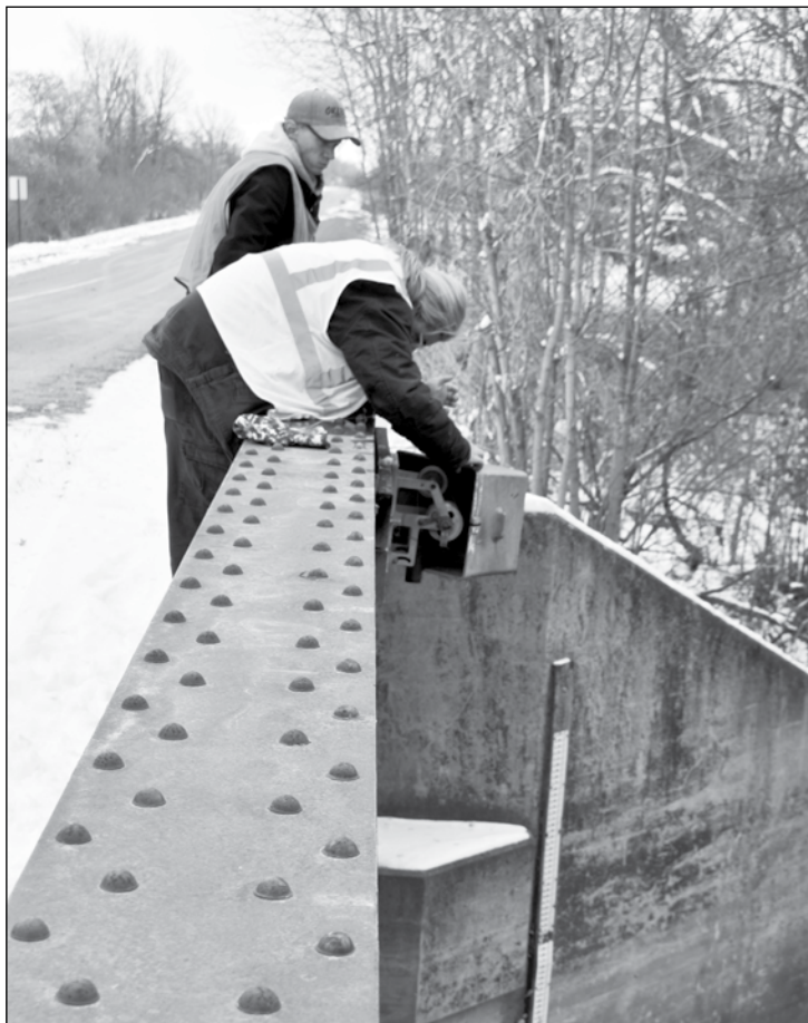
Ruben Osborn and Peyton O'Neill are doing the tape-down: they are measuring the height of the bridge to the top of the water
