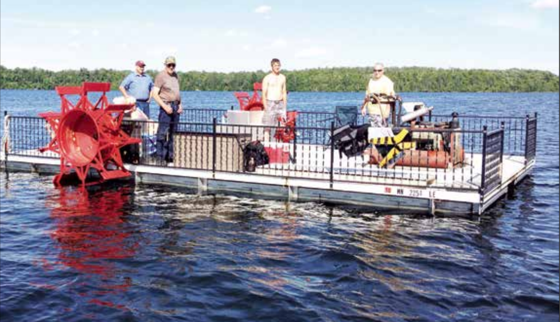
It's a raft, It's a Barge, It's a Boat? Gary Matthis of Hangaard Township (north of Gonvick) has been farming all his life and has had to innovate and rebuild lots of machinery to get the job done. Now, just for fun, he has built a paddle boat for use on local lakes. The deck is 16 1/2x28 1/2 ft. with pontoons for flotation. The motor is a stationary Wisconsin engine that drives the 2 paddle wheels. The paddle wheels are made of tractor rims with the paddles welded in place. This photo was taken on Clearwater Lake on Sunday afternoon with Gary, his family and friends, enjoying a beautiful Minnesota summer day.
