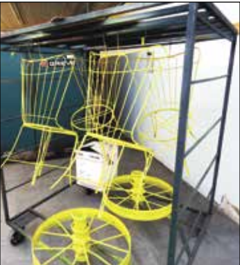
After the powder coating process, articles such as metal lawn furniture need to cure on racks.
