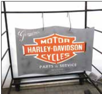
To make different colors, each segment has to be taped off with the color applied and then the next color. This sign has only the first color applied.
