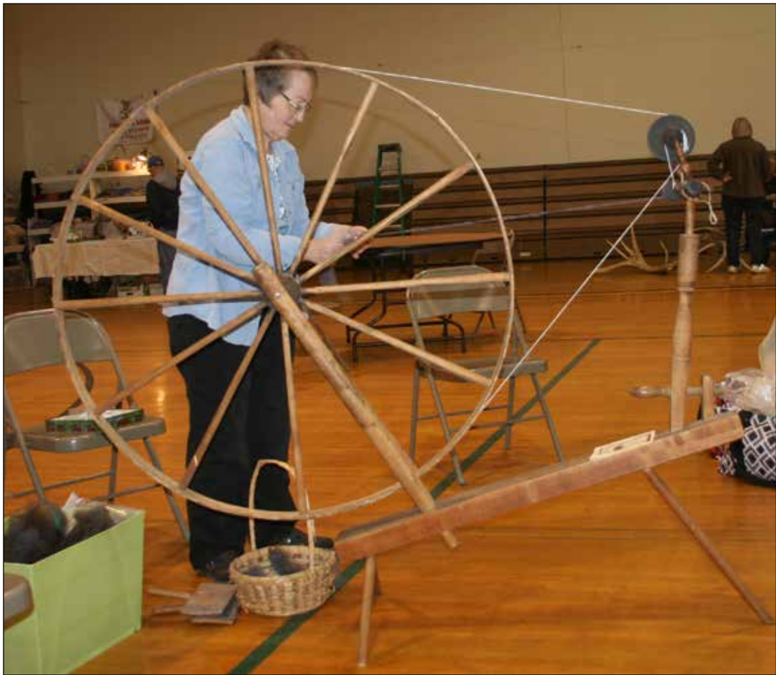
Rilla Nelson of Clearbrook brought her great-great-grandmother's spinning wheel to the Farm to Fiber Festival. Known as a great wheel, wool wheel, or walking wheel, this large spinning wheel was made in England. The spinner must stand to operate this wheel, due to its large size. Rilla was one of many exhibitors who demonstrated a variety of skills needed in the process of creating fabric items from wool. See story on the Canary front page.
