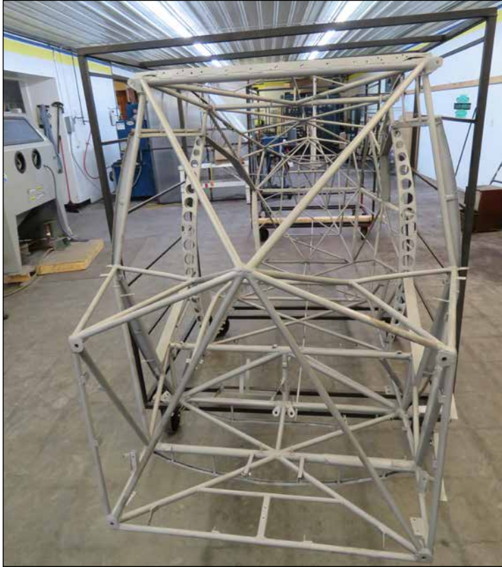
A front view of the airplane frame that is getting prepared to be put in the powder coating oven.
