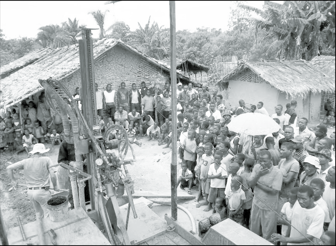
Congo Frontline Missions drills with a Little Beaver LS200H portable rig in Obilo, a village in the Democratic Republic of the Congo in June 2012. The drilling formation was sand. Photo courtesy of Congo Frontline Missions.
