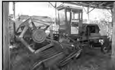
Versatile mod 400 18' self propelled swather, hydrostatic
