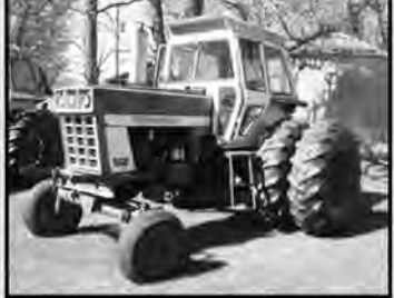
1973 IH 966 diesel tractor w/cab, dual 18.4-34 rubber, 3pt, single hyd, 540/1000 PTO ser # 2510175U022492
