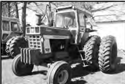
1974 IH 1066 Turbo Diesel tractor w/cab, suitcase weights, 3 pt, fair 18.4-38 hub duals, wheel weights, dual hyd, 540/1000 PTO , 3pt. ser# 2510175U022492
