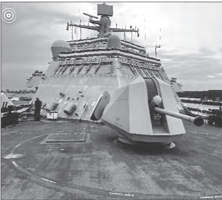
The flight deck on the USS Minneapolis-Saint Paul LCS 21 is more than 1.5 times larger than most U.S. Navy surface combatants. Three reconfigurable spaces allow for flexible armament including guns and missiles.
