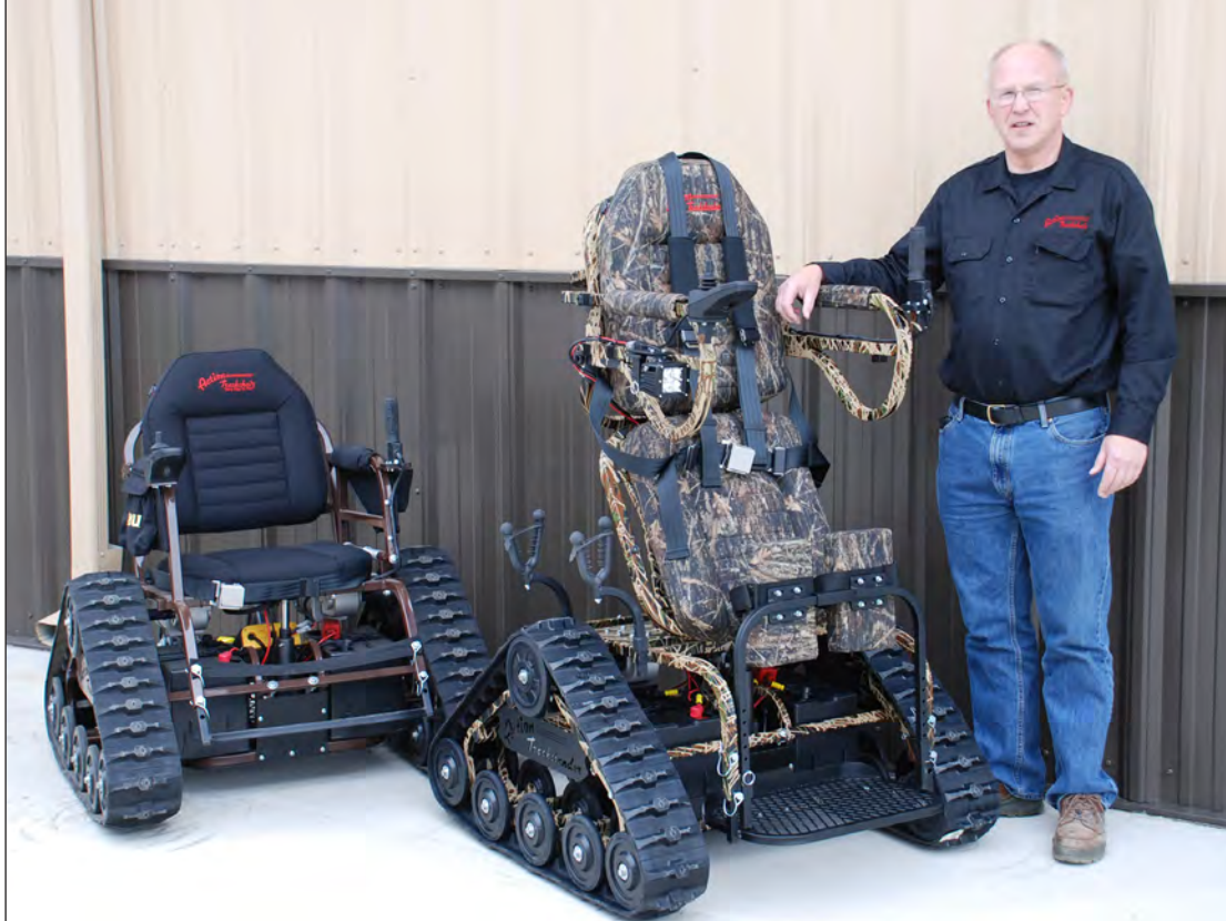
Tim Swenson, founder of Action Manufacturing, developed two models of his tracked chair for going nearly anywhere—through sand and mud, up and down hills, and over snow and ice. The range is up to 5 miles, depending on conditions.
