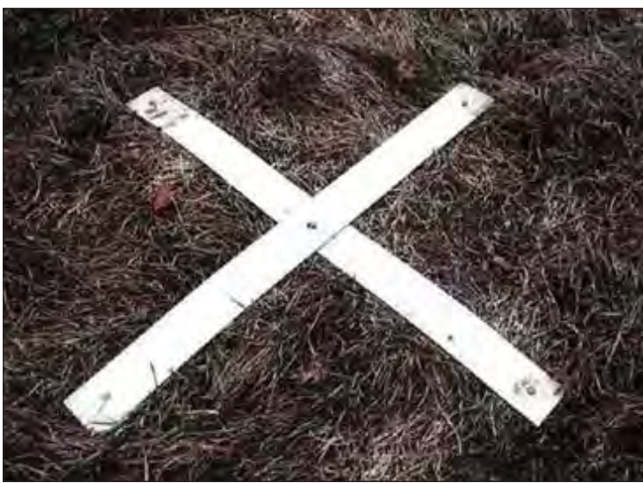
The photos are examples of aerial photography targets used in previous MnDOT projects. Targets for this project may differ in appearance.
