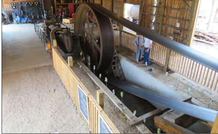
This is the huge pulley drive for the Redby Mill (steam driven).
