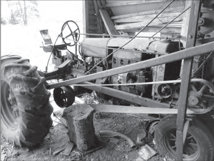
Here is an F-20 I came across last summer near Menahga. It had a mechanical loader run by the belt pulley!
